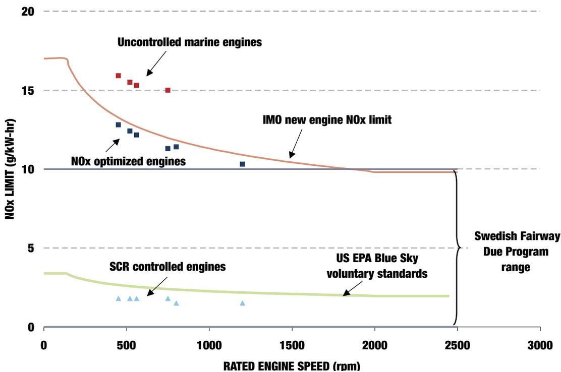
FIGURE 14. Marine Engine NO<sub>x</sub> Standards in the United States, EU, and Sweden (Eyring 2005a, SMA 2005)
